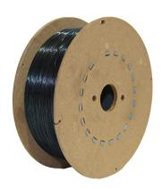
Tru-Core<sup>®</sup> MC 110C-K4 is a low alloy steel, metal cored electrode for gas shielded arc welding of low alloy, and carbon steels requiring tensile strengths exceeding 110 ksi and excellent CVN values, even in freezing temperatures as low as -60°F. It is suitable for both single and multiple pass applications with fillet or groove welds.
